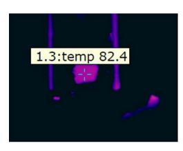
Thermogram 1.4 shows the target after recalibration of the imager to the degraded  $\tau$  value of the CaF2 Test Window. Transmittance was adjusted to 15% to bring the apparent temperature in line with the true temperature. This represents a 69.4% degradation in transmission of the CaF2 Test Window over a two (2) year period.
