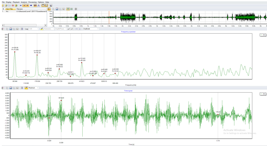
Figure 10 Ultrasound software picking up Arcing fault
